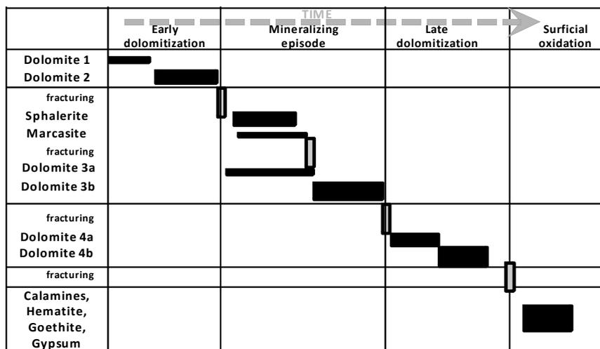
fig 2. Paragenetic sequence of the Zn-mineralization and the associated dolomitization in the Río Mundo
